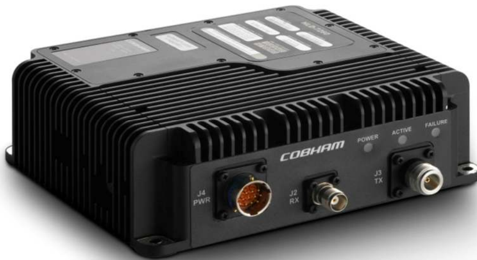
Figure 4-6: HLD-7260 High Power/Low Noise Amplifier and Diplexer
