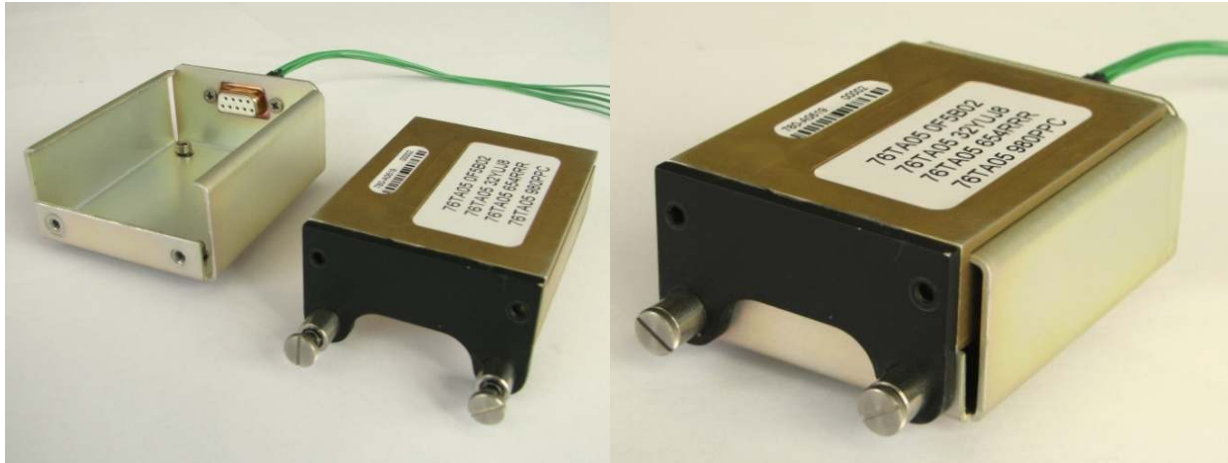
Figure 4-3: External Configuration Module holder.
